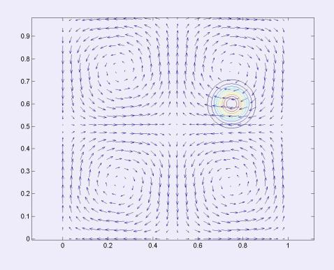
$$\frac{\partial C}{\partial t} + a^x \frac{\partial C}{\partial x} + a^y \frac{\partial C}{\partial y} = 0$$
